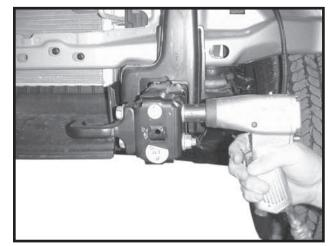
6. Remove tow hooks (if equipped) by removing two bolts on each side, bolts and tow hooks will not be reused (holes may need to be drilled for some models).
